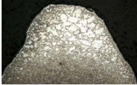
**Figure 1-35** Gross decarburization in a steel fastener.
