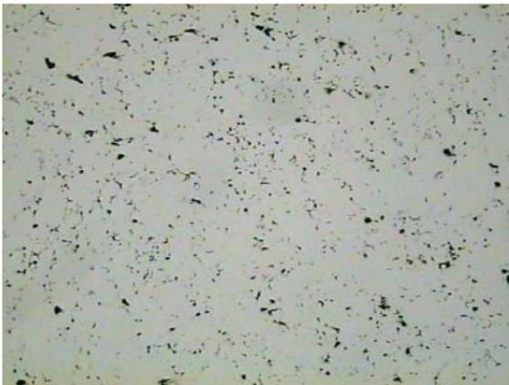
**Figure 11-26** Sintered Iron, Mag. 100X (B.F.), as polished.
