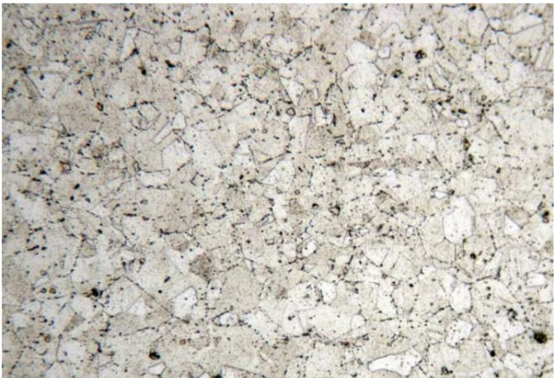
**Figure 11-46** Wrought nickel, 200X (BF), Etchant HCl and H<sub>2</sub>O<sub>2</sub>.
