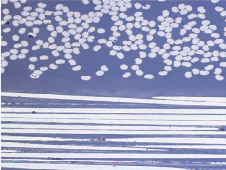
**Figure 11-18a** Carbon fibers in polymer matrix, 400X, as polished.
