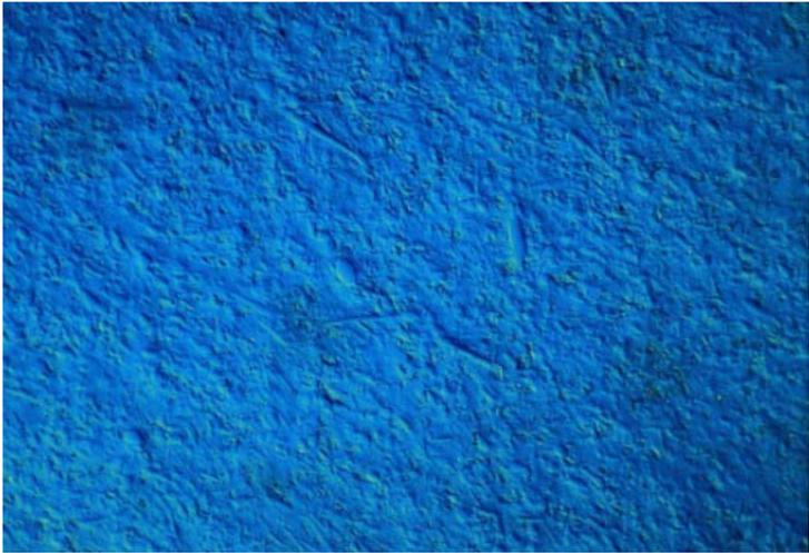
**Figure 11-61a** ZrB<sub>2</sub> particles in a Titanium Matrix, 1000X (DIC), as polished.
