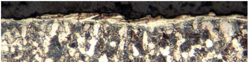
**Figure 1-31** Cracks in recast layer.
