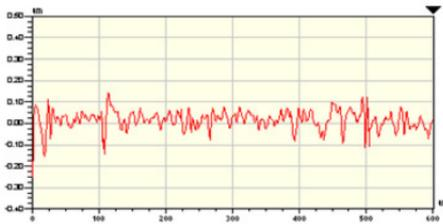
Surface roughness of a low carbon steel polished with 3 μm polycrystalline diamond
