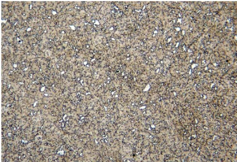
**Figure 11-41d** 400 Series Stainless Steel, 200X (BF), Etchant Viella's.
