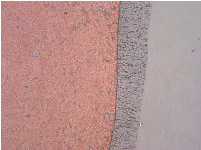
**Figure 11-9** Diffusion of Stainless Steel (gray) into copper, 200X B.F., (as polished).
