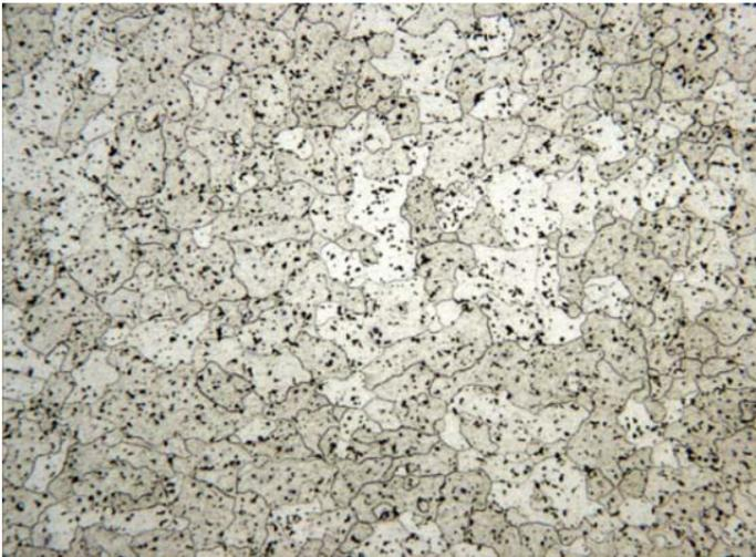
**Figure 11-6** 6061 aluminum, Kellers reagent, 200X.
