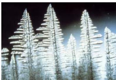
**Figure 1-13** Dendrite treelike structure.
