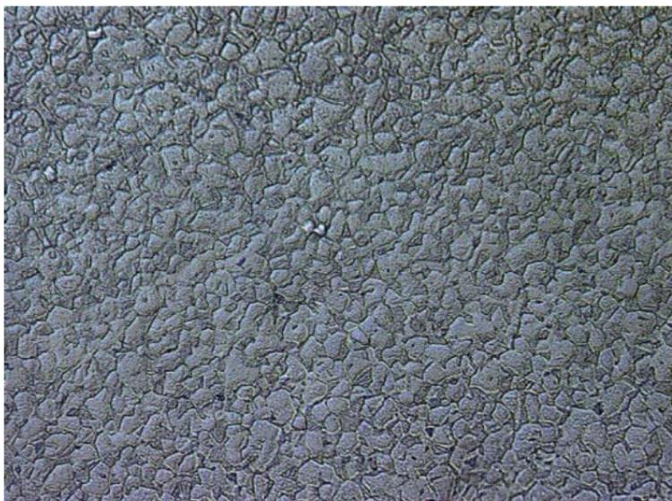
**Figure 11-47** Ti<sub>6</sub>Al<sub>4</sub>V Titanium Alloy, 400X (DIC), Etchant Kroll's Reagent.
