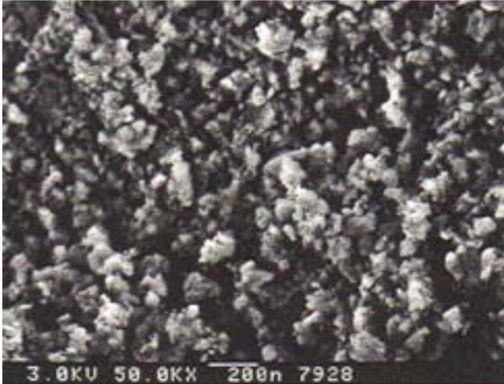
**Figure 6-2** 0.05 micron polycrystalline alumina.
