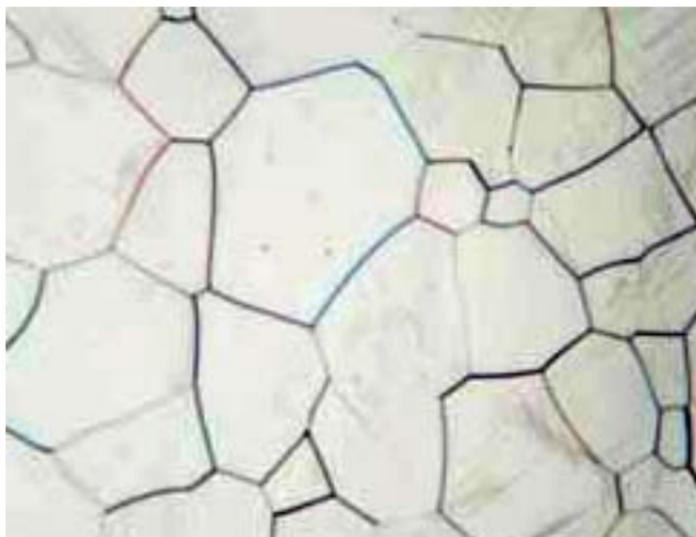
**Figure 11-34** GaAs, etched with HOCl-, mag. 1000X, DIC.
