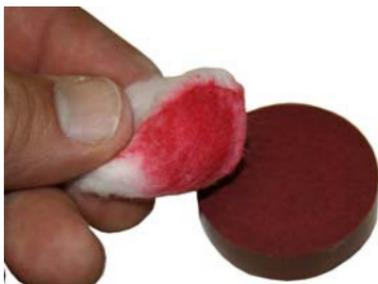
**Figure 4-17** Insufficient curing of phenolic resin causes alcohol to dissolve the dye.
