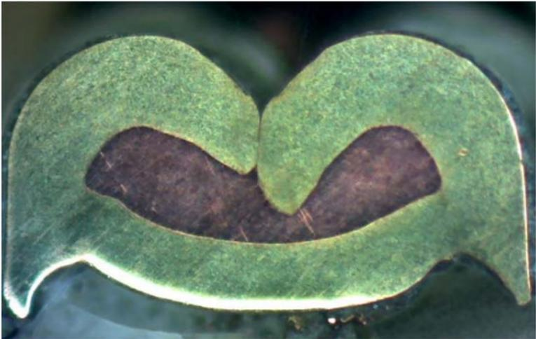
**Figure 11-10b** Proper crimping of copper wires.
