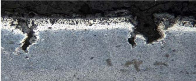
**Figure 1-15** Intergranular alloy depletion in nickel.
