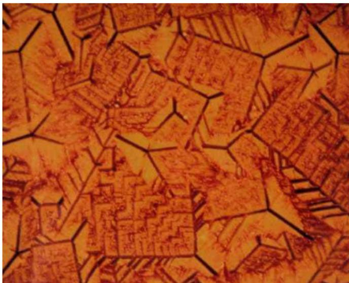
**Figure 11-78** Alumino-silicate glass, 400X (Polarized light), as polished.
