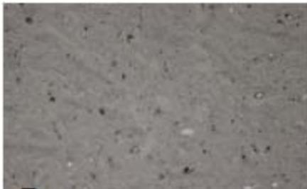
**Figure 4-13** Glass-filled epoxy resin, 100X.
