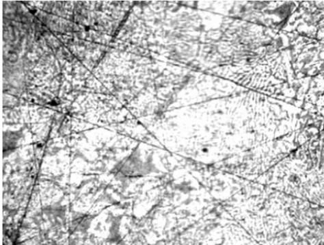
**Figure 6-16a** Bismuth-tin alloy prior to polish-etch-polish.
