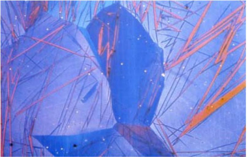
**Figure 11-44** Fe-Ni-Co-Al Alloy, 400X (Polarized Light).
