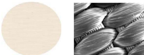
**Figure 5-29** POLYPAD polishing pad and SEM image of fibers.
