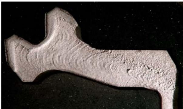
**Figure 1-40** Improper flow line direction normal to maximum stress, Etchant HCl+H<sub>2</sub>O<sub>2</sub>.
