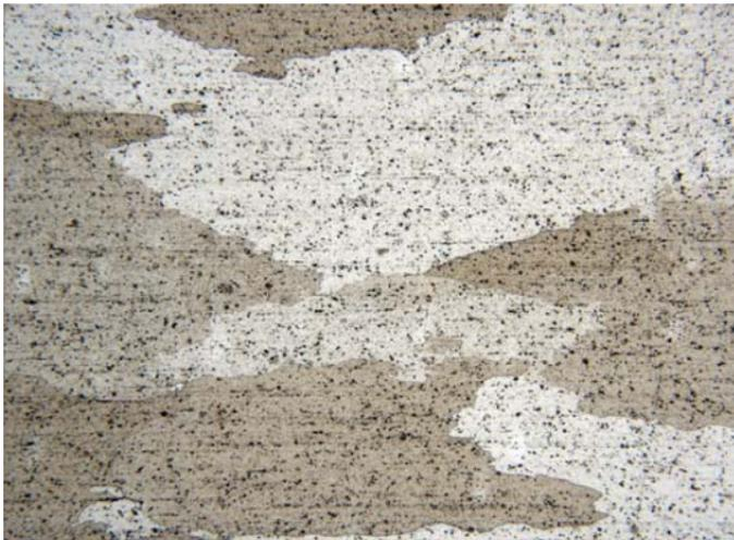
**Figure 11-7** 7075 aluminum, Kellers reagent, 200X.
