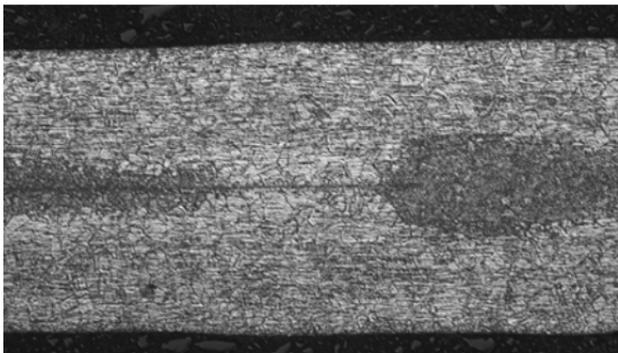
**Figure 1-23b** Discontinuous seam weld with poor penetration.
