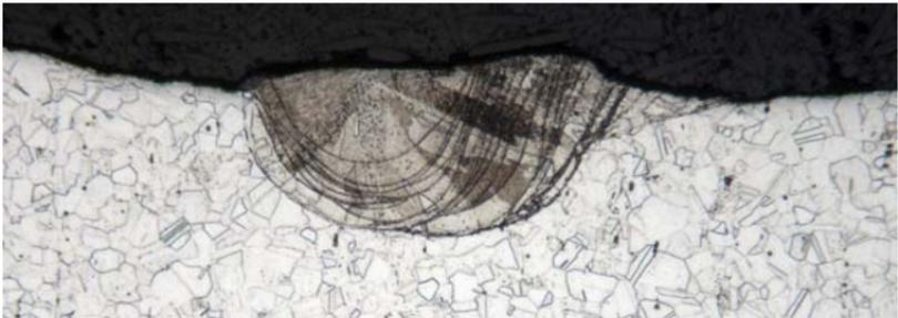
**Figure 1-30** Localized recast layer.
