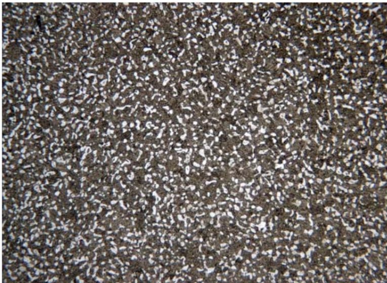
**Figure 11-49** Wrought Titanium, 200X (BF), Etchant Ammonium Bifluoride.
