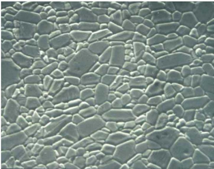
**Figure 11-67** Alumina, 5,000X, Thermally etched.
