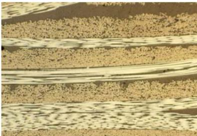
**Figure 1-25** Carbon fiber composite.
