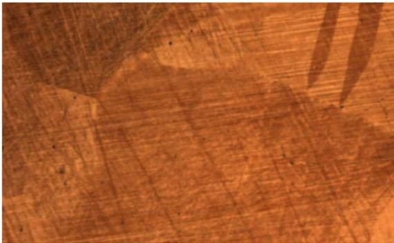
**Figure 6-13b** Tin after attack polishing with 2% Nital, mag. 50X.
