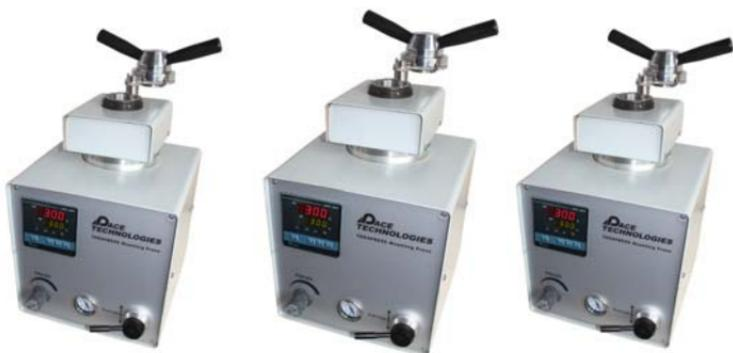
**Figure 4-10** Compression Mounting Press.
