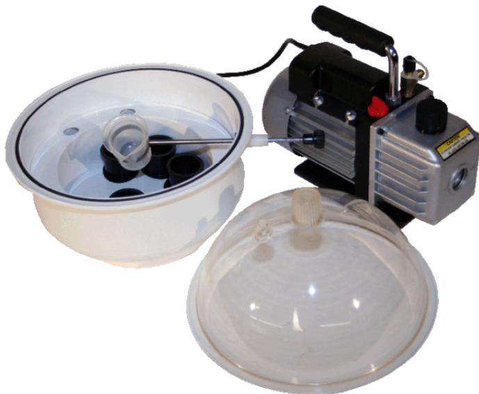
**Figure 4-5** Vacuum impregnation device.
