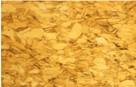
**Figure 11-11b** 70-30 Brass cold rolled, 200X (B.F.),
