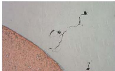
**Figure 1-8** Welding crack in a copper-stainless steel weld.
