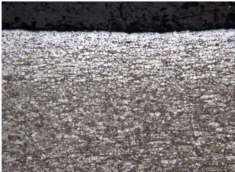
**Figure 11-50** Alpha-rich Case Wrought Titanium, 200X (BF).
