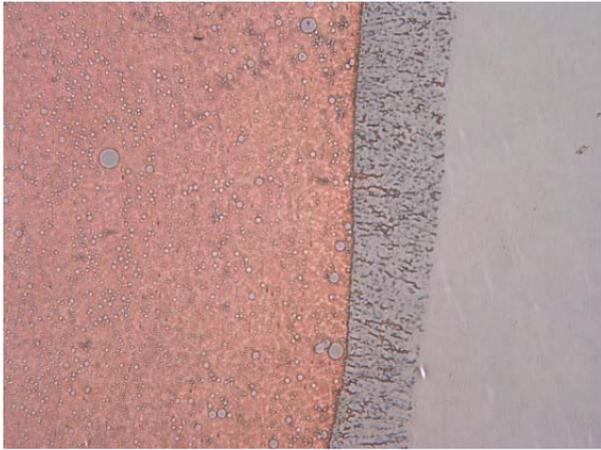
**Figure 1-22** Copper-stainless steel weld diffusion of the stainless steel into the copper
