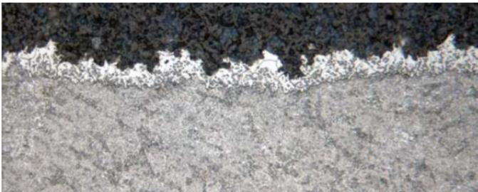
**Figure 1-16** Intergranular attack in nickel.
