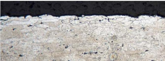
**Figure 1-17** Intergranular cracking in aluminum.
