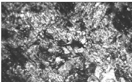
**Figure 4-14** Conductive graphite mount, 100X.
