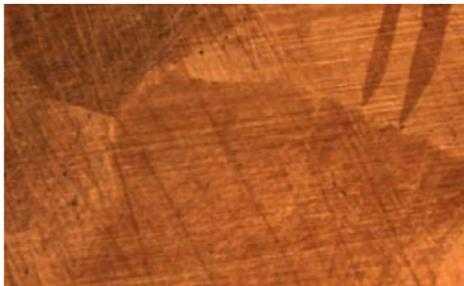
**Figure 6-18b** Large tin grains following attack polishing with 2% Nital.
