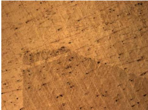
**Figure 6-13a** Tin with embedded abrasives, mag. 50X.
